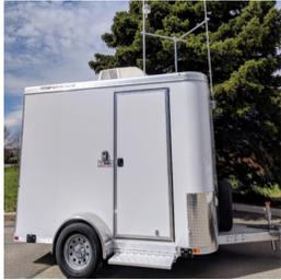
**RHyNO (Real-Time Hydrocarbon NOx) Trailer:** Crestone designed and built a custom air quality station to more efficiently monitor air quality during each phase of operations. The mobile trailer measures air pollutants and meteorological conditions (wind speed and ambient temperature) at production sites to evaluate air quality and determine if adjustments are necessary.
